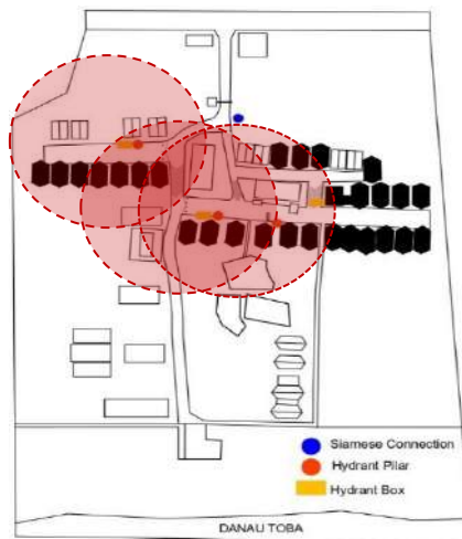
Gambar 5.11 Analisa jarak radius hydrant
